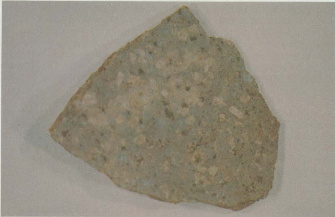
Fig. 5. Photograph showing the two distinct sizes of K-feldspar in alkali granite (photo by the author, ASA 100).
