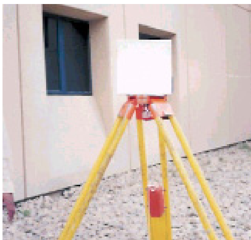
Fig. 13. The smooth white porcelain tile reflector.
