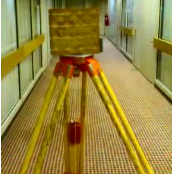
Fig. 18. The brown mud sheet reflector.
