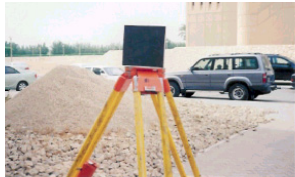
Fig. 14. The smooth black porcelain tile reflector.
