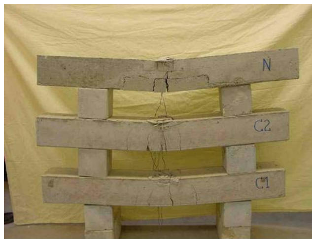
Fig. 17. Control and tension side concrete (N) repaired specimens.
