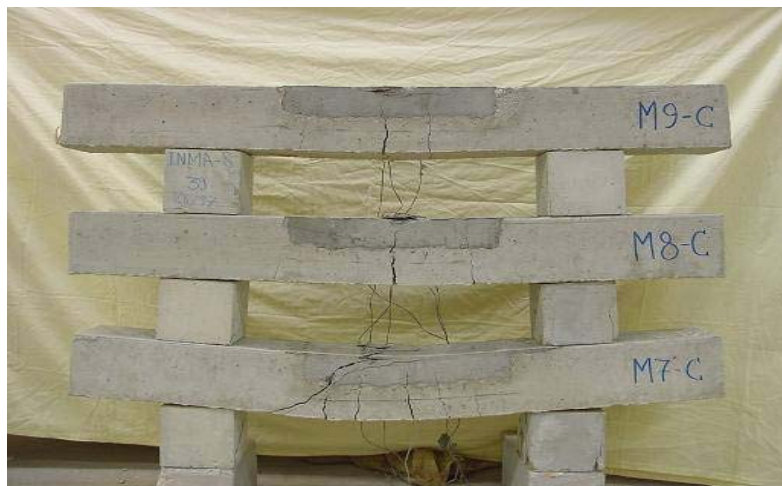
Fig. 19. Beams repaired in Compression with M7, M8 and M9 materials.
