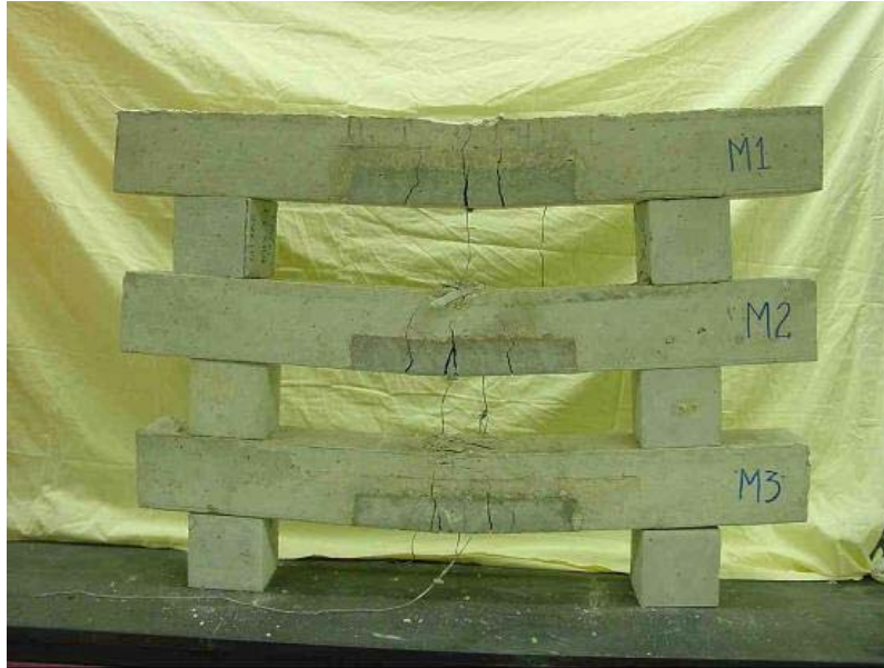
Fig. 18. Beams repaired in Tension with M1, M2 and M3 materials.
