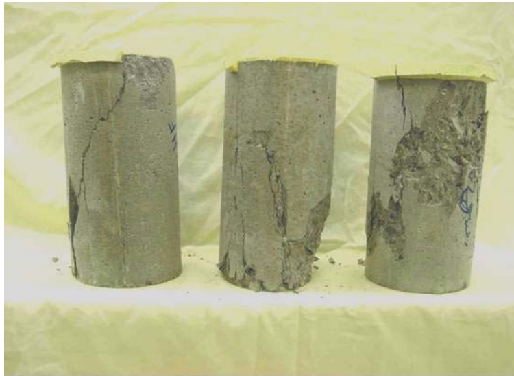
Fig. 1. Typical failure cracking pattern of some of the tested cylinders.
