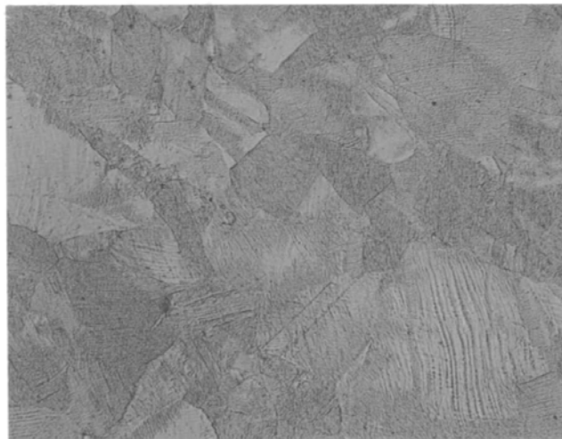
Fig. 8. Microstructure of 70:30 brass after the reverse shear cycle, at a total accumulated plastic shear strain of 1.6.
