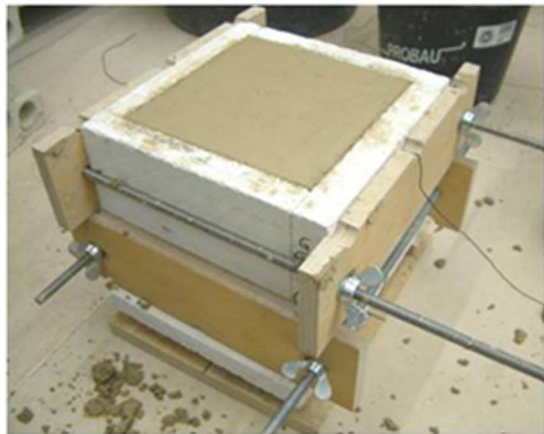
c) The Protection Cover after filling it up with the loam of the sample
